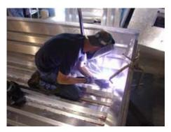
The backbone of each Xpress boat is its longitudinal rib system. Each rib receives over 200 individual welds, making all Xpress aluminum hulls unequalled in strength and rigidity.
