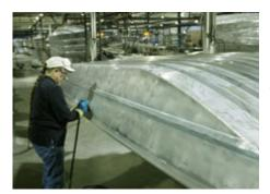
Any imperfections found on the hull are buffed out before beginning the paint process.
