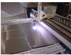
Each part is designed using a CAD program. After the aluminum is fed through the decoiler, it is cut with a plasma torch. This state of the art process ensures each part is made to exact specifications.
