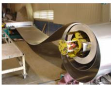
Xpress Boats are constructed with quality .080-.125 gauge aluminum alloy. The aluminum is fed through a decoiler to prepare it for cutting.
