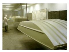
Each hull undergoes a spray on paint process using high quality acrylathene enamel paint. This high gloss paint is often mistaken for those used on fiberglass boats.
